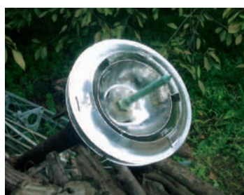
Radioactive lightning conductor
